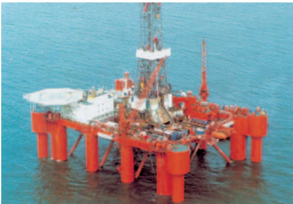
Semi-submersible drilling rig
