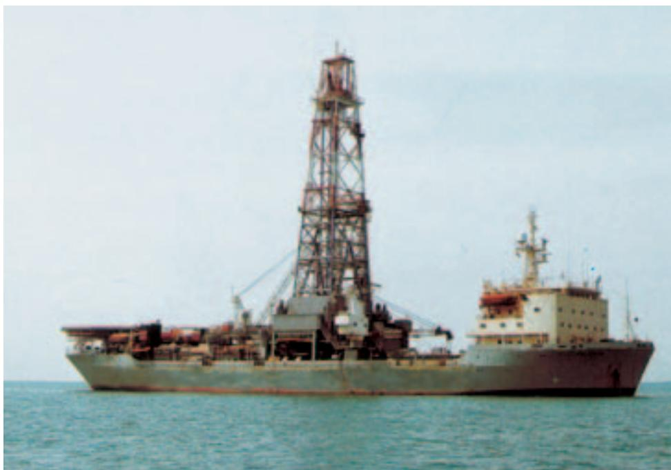
Dynamically positioned drillship
